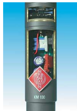
Section of Capsule with Hybrid Module Visible
